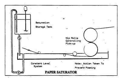
The saturated paper should be fed from the saturator to the drier in such a way as to provide minimum tension to the paper, in order to maintain the crepe, then rapid drying applied, as for example with infra-reds, to rapidly reduce the water content of the paper,
