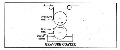
coating. A doctor blade is necessary to remove excess coating from the gravure roll. Though time, the gravure roller will wear, and there are commercial kits available to measure the degree of wear, by taking an impression of the roll.
