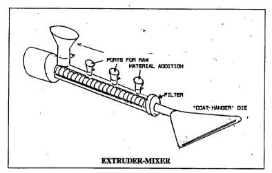
The latest technique for hot melt adhesive systems is the use of an <u>extruder</u>, with feed ports for the various ingredients, this having the advantage of a continuous mixing system, which can be terminated at any time, with no residual adhesive batch to deal with. In some machines, known as a <u>pultruder</u> the extruder screw, of a special design, both rotates and cycles back and forth, for better mixing.
