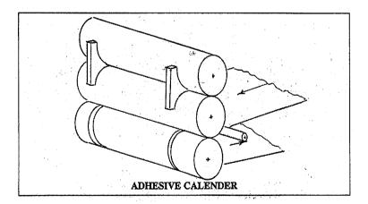
The pre-heated adhesive is placed between the top and middle rolls, the gap between the two determining the adhesive coating weight, which adheres preferentially to the middle cooler roll. The tape base to be coated passes around the bottom roll, and is brought into
