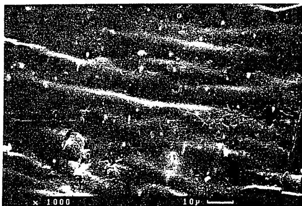
Figure 3. Magnified view of tape surface, photographed using a scanning electron microscope (carbon coating; tape ex 2490/81).
